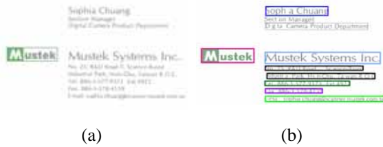
Fig. 8 An example of experimental results of text line classification in an English name card image. (a) The original image. (b) The resulting image after text line classification.
