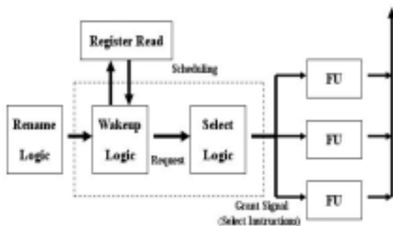
Figure 2.2: Conventional Execution Core
