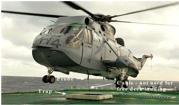
Figure 2. Rapid Assist Securing and Traversing System (The Trap)[2]
