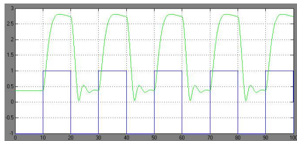
Fig. 2. The square wave (lower) as test pattern and the output responding curve (upper) of the nonlinear plant.
