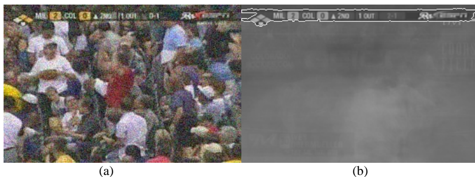
Fig. 7. (a) A noisy and complex-background video frame; (b) a detected caption region in the averaged video frame.
