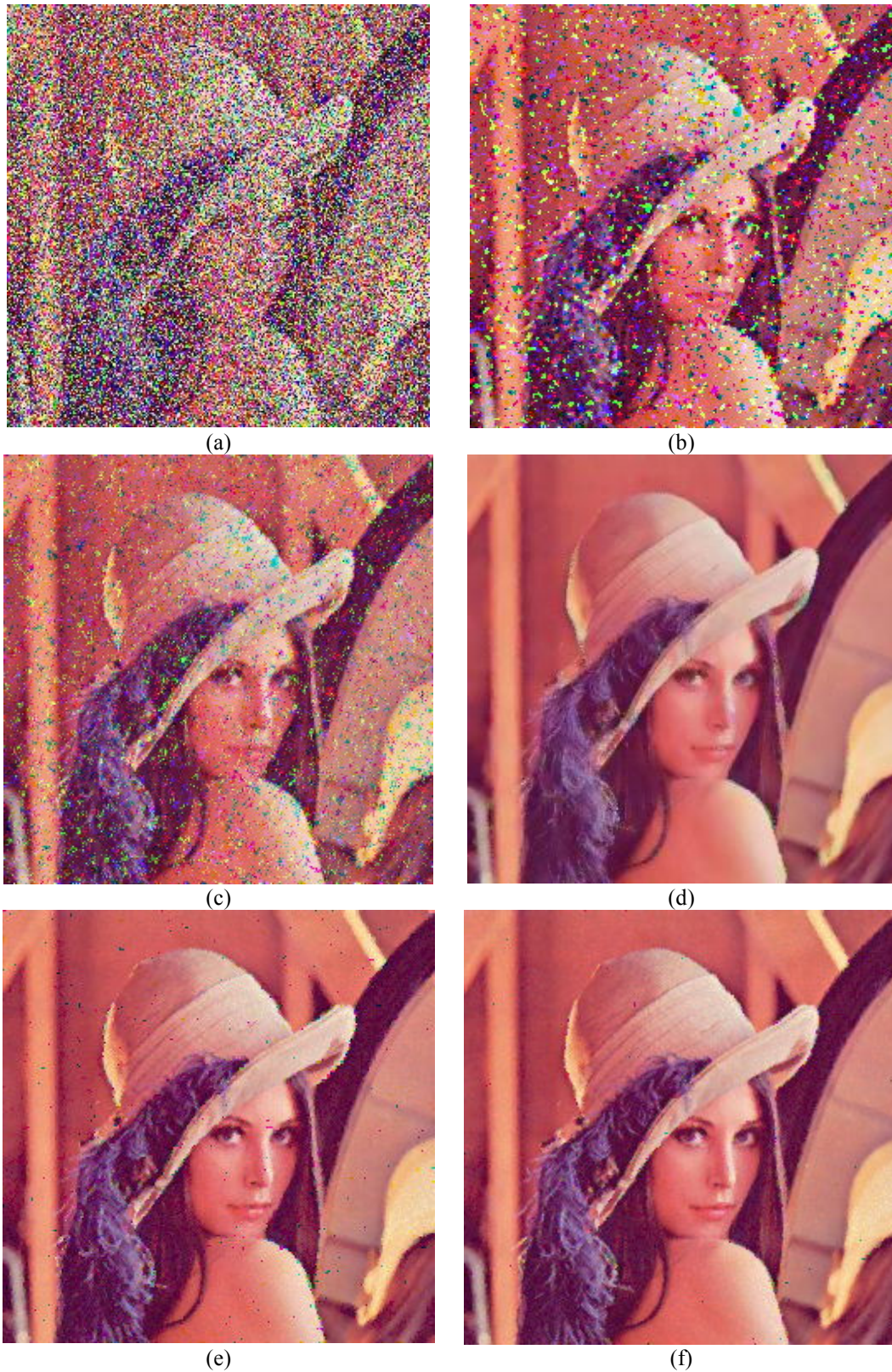
Fig. 22. (a) Noisy color image “Lena” corrupted with 50% noise rate, and the results of denoising corrupted image using the (b) EIDA filter, (c) Russo filter, (d) SMF filter, (e) MGFF filter, and (f) OIA
