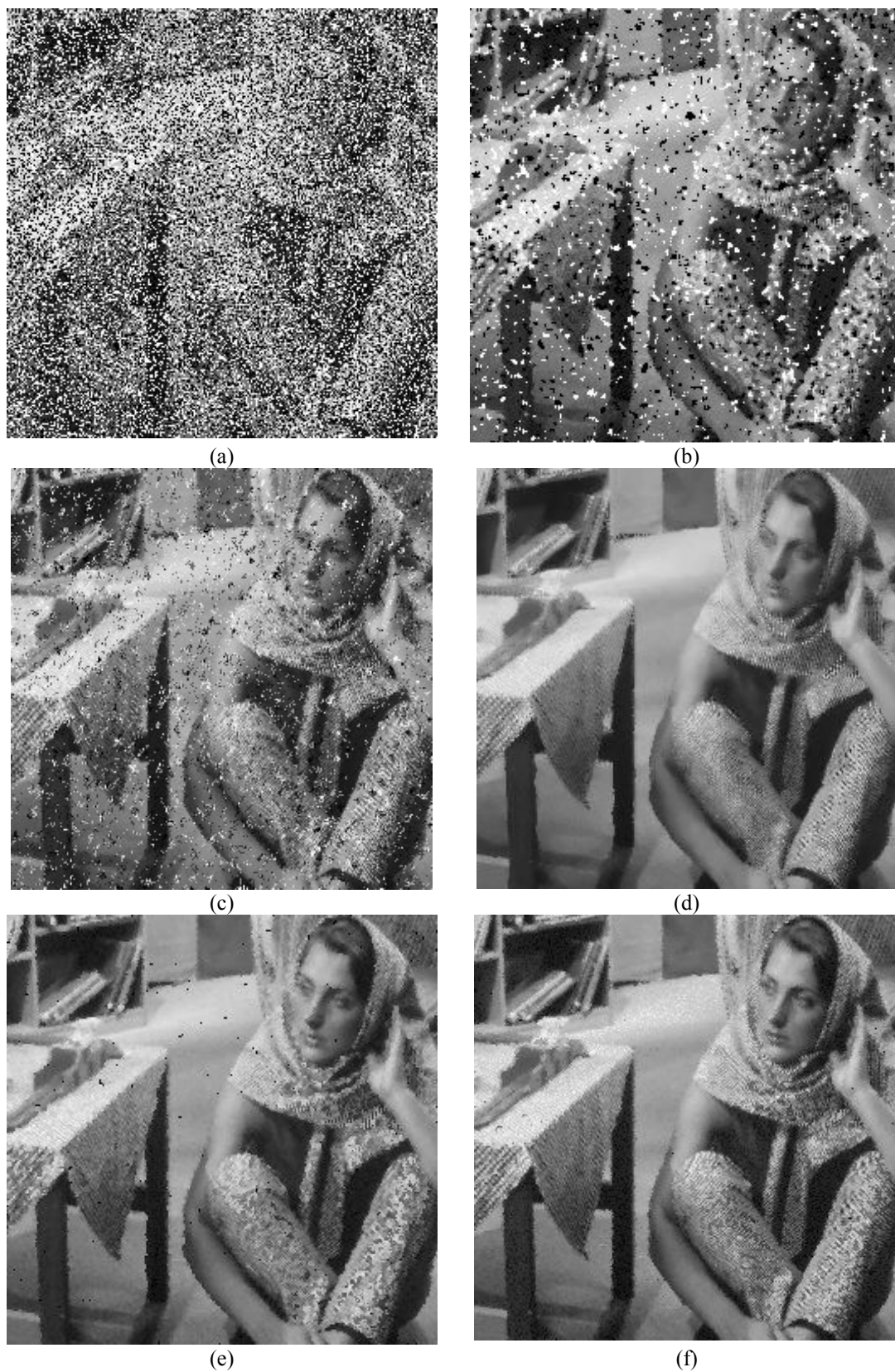
Fig. 10. (a) Noisy gray image “Barbara” corrupted with 50% noise rate, and the results of denoising corrupted image using the (b) EIDA filter, (c) Russo filter, (d) SMF filter, (e) GFIF filter, and (f) OIA
