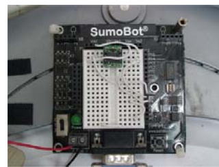
Figure 3. BS2 IC and digital compass
