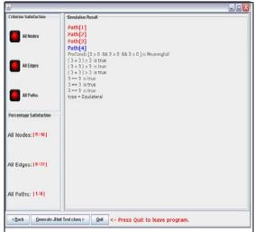
Figure 5. The expected output and coverage criteria satisfaction rates for fourth test path of the triangle problem.
