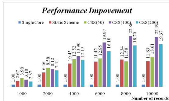
Figure 6. The performance comparison of different load balancing schemes by using 8 processor cores
