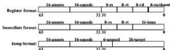
Figure 9: Three instruction formats that SimAsync supports.
