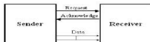
Figure 1: Control signal lines and Data wires between two stages in micropipeline.
