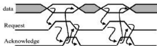
Figure 6: Four-phase data-bundled communication used by AMULET 2. Notice that we need to restore the control signals to the steady state after data transfer.
