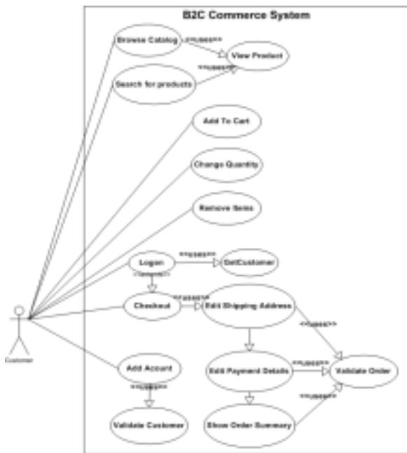
Figure 7. Use Case Diagram for B2C EC Domain
