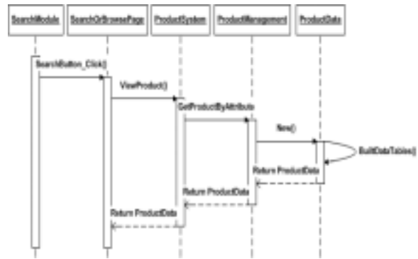
Figure 12. Sequence Diagram for Use Case Search for Products
