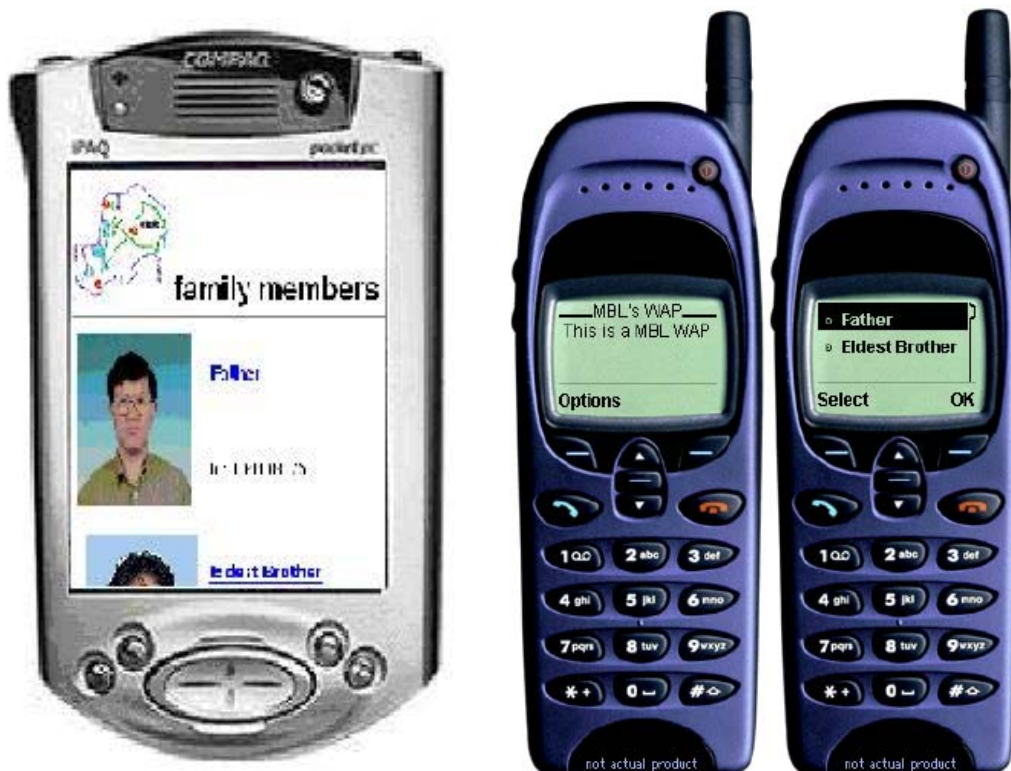
Fig. 5. A screenshot of Compaq iPAQ H3800 Pocket PC with 11 Mbps wireless connection and screenshots of WAP mobile devices with 9.6 Kbps dial up connection.
