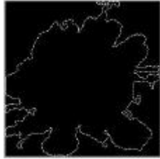
Figure 10 The reconstructed image of Fig. 6 by Fourier descriptors.
