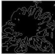
Figure 4 The resulting image from Fig 3 after morphological dilation, median filtering, and boundary extraction.
