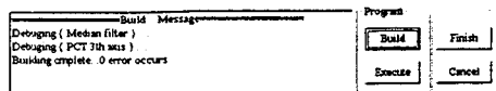
Fig. 4 After pressing button "Build" VPW will check if the linkage is legal. This is a legal one.
