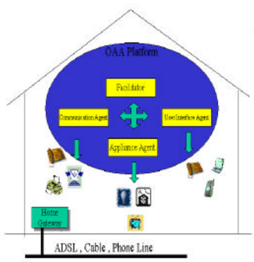
Figure 2: Architecture of home automation system
