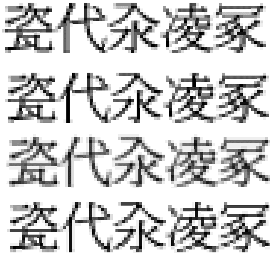
Fig.5. Comparison of the filtered characters: the top line denotes the grayscale character without grid-fitting; the second uses Box filter after grid-fitting; the last uses Gaussian filter after grid-fitting.
