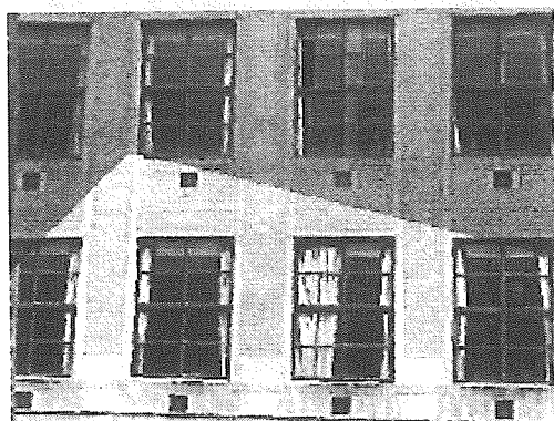
Photo.2 Part of the environment map generated by ordinary ray-casting. There is obvious intensity discontinuity.
