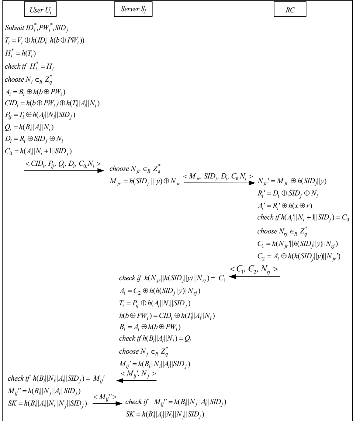
Fig.1. the login, mutual authentication and key agreement phases of Hsiang-Shih scheme
