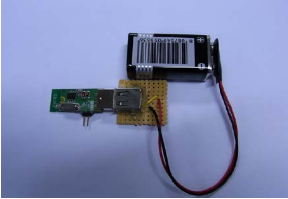
Figure 2: Beacon source powered by a 9-volt battery
