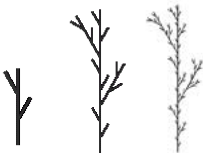
Figure 4. L-system plant with rule string substitution 1 times (left), 2 times (middle) and 3 times (right)
