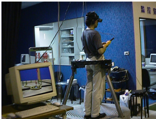
Figure 15. A trainee is immersed in the overhead crane training system
