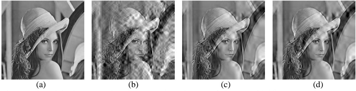
Fig. 10. The original, corrupted, and processed test images of “lenna” with bit rate = 0.4bpp, BER = 0.1%, N_{ave} = 2 , and errors occur in LH_1 , and HH_1 : (a) the original image (PSNR = 36.14dB); (b) the corrupted image (PSNR = 21.02dB); (c)-(d) the processed image by the zero-substitution approach (PSNR = 22.82dB) and by the proposed concealment approach (PSNR = 26.30dB).
