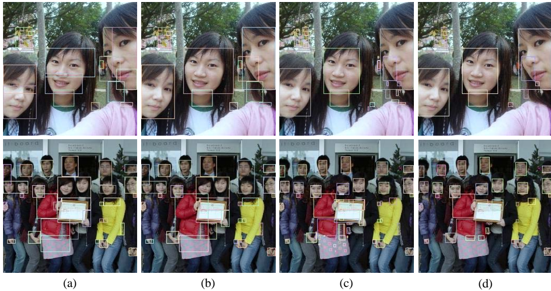
Fig 2. A sample test for candidate face regions. (a) The result by clustering algorithm; (b) The performance after frame integration algorithm; (c) Processing by frame segmentation algorithm; (d) The final result after forsaking the unlikely regions.
