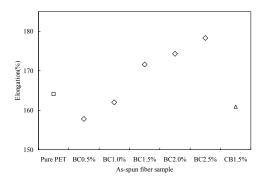
Fig. 4. Elongation of as-spun fiber sample (BC: Bamboo Charcoal; CB: Carbon black)
