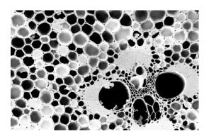
Fig. 1. The multi-porous structure of bamboo charcoal (Magnification: 500×)
