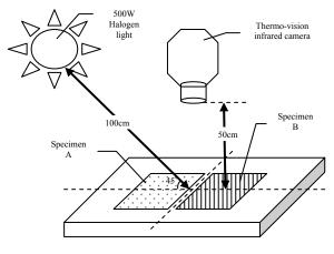
Fig. 2. Scheme of testing elements for heat preservation analysis
