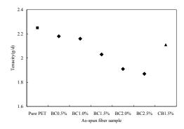
Fig. 3. Tenacity of as-spun fiber sample (BC: Bamboo Charcoal; CB: Carbon black)
