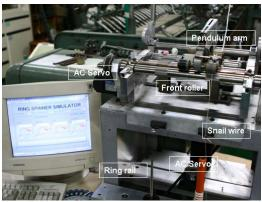
Fig. 1 Experimental ring spinning system
