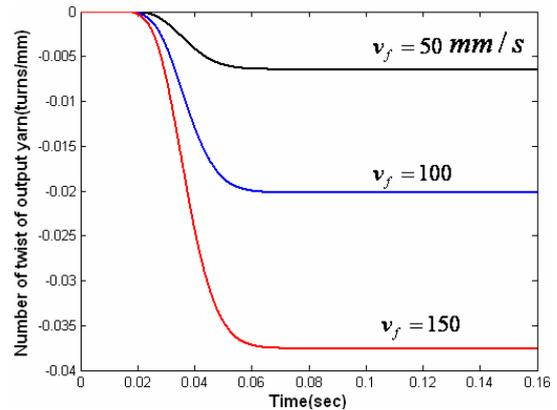
Fig.10 Response of the twists of output bundle to step input thickness.
