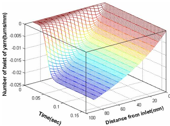
Fig.8 Response of the twists of in-process bundle to step input thickness.
