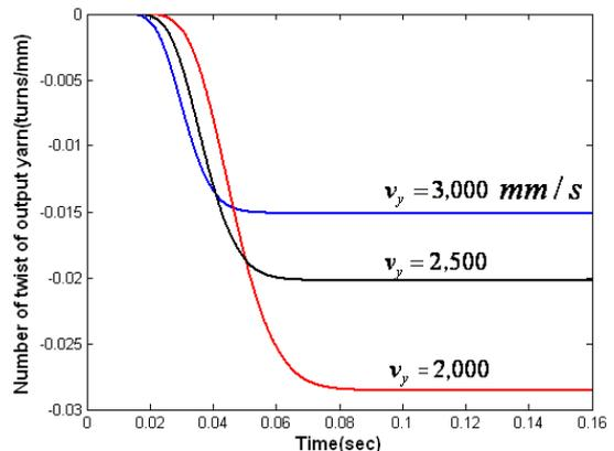
Fig.11 Response of the twists of in-process bundle to the step change of the yarn delivery speed.
