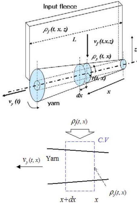
Fig.2 Infinitesimal yarn section in friction spinning.
