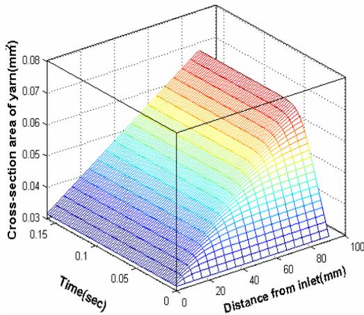
Fig.6 Response of cross-sectional area of in-process bundle to step input thickness.
