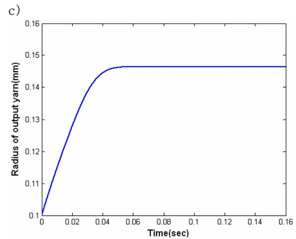
Fig.7 Response of the in-process bundle for a step input of the fleece
