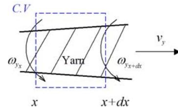
Fig.3 The twisting model of a yarn
