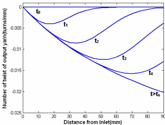
Fig.9 Transient behavior of the in-process bundle twists at various time points for a step input thickness.
