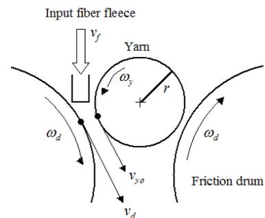
Fig.1 Schematic representation of the friction yarn formation.
