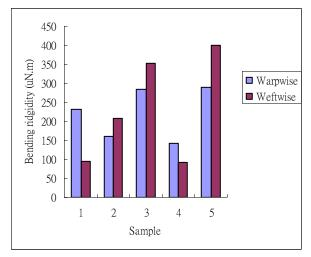
Fig. 4. Bending rigidity of spacer samples
