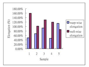
Fig. 5. Elongation of different spacer samples
