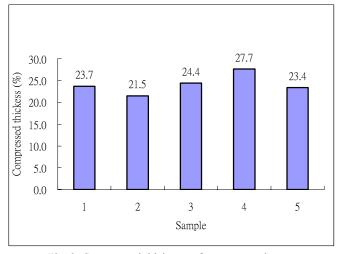
Fig. 3. Compressed thickness of spacer samples
