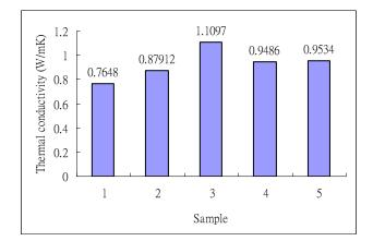
Fig. 2. Thermal conductivity values of different spacer fabrics
