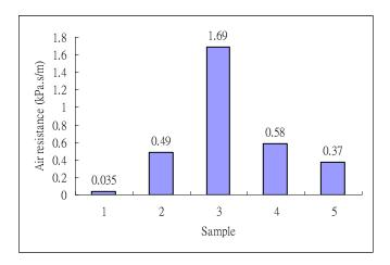
Fig. 1. Air resistance of different spacer fabrics
