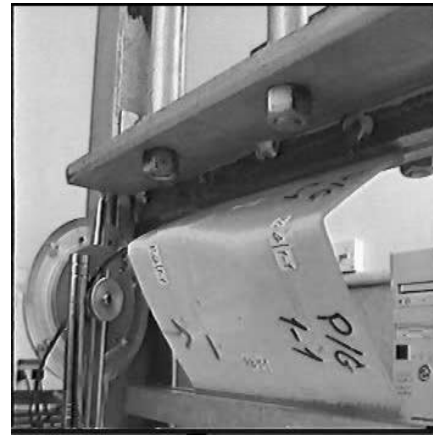
Fig. 5. A Polyester-Glass fabric and Polyester resin composite plate after final damage
