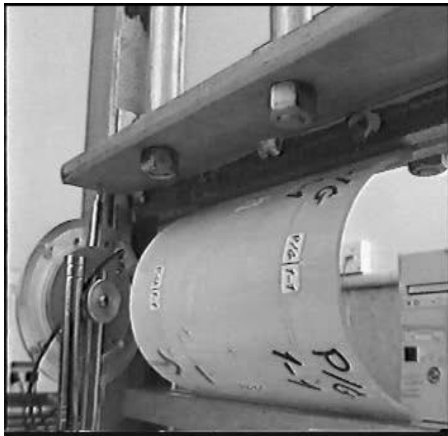
Fig. 4. A Polyester-Glass fabric and Polyester resin composite plate under buckling test
